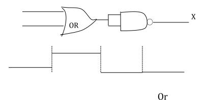
Two car garages have a common gate which needs to open automatically when a car enters either of the garages or car enters both. Design a truth table, logic symbol and hence Boolean expression for a circuit that resembles this situation using diodes.
