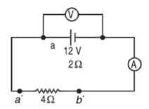
15. In the circuit shown, the reading of voltmeter is 20V. Calculate resistance of voltmeter. What will be the reading of voltmeter if this is put across 200Ω resistance?
