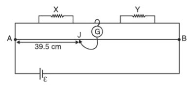
A meterbridge is in balance condition. Now if galvanometer and cell are interchanged, the galvanometer shows no deflection. Give reason.
